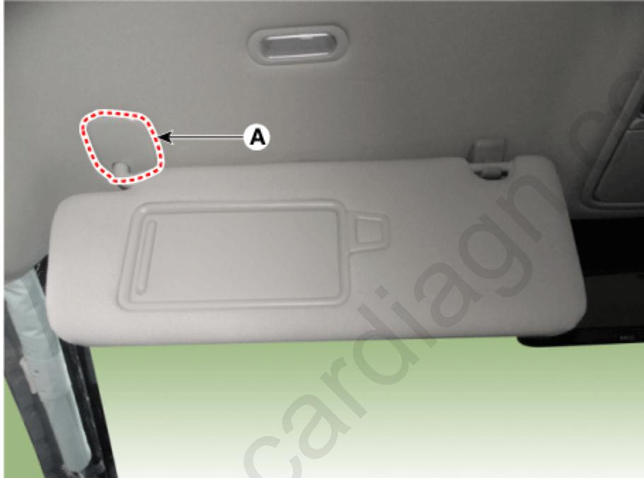
2. Separate the sunvisor (A) after loosening the mounting screw.
