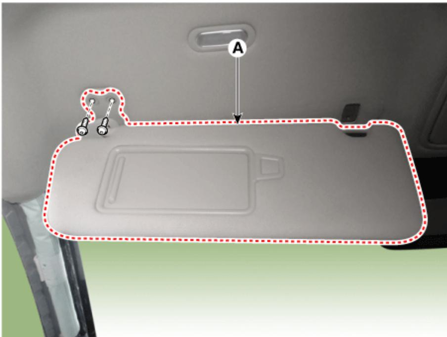
3. Remove the sunvisor after disconnect the connector (A).
